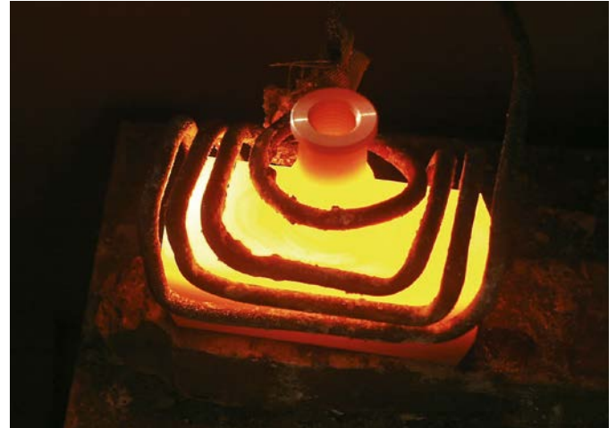
optris® CTlaser 1M/2M/3M devices used during induction-hardening
