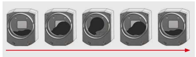
To enable offset referencing, the whole field of view of an infrared sensor array is closed for a brief period
