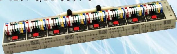
\*Since this bridge box is [ the shield (E terminal) ] common, only when connecting DPM-911B/912B / two or more 913B, a shield exchange cable (N-117) is needed for each channel.
