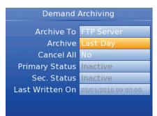
Set up the PC as a server as described in the User Guide HA030554 Appendix C. Connect the destination PC to the instrument using the ethernet RJ45 connector.
