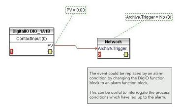
When the event occurs data is automatically transferred to the memory stick. This can be seen in Demand Archiving under Status → Complete → Transferring → Complete.
