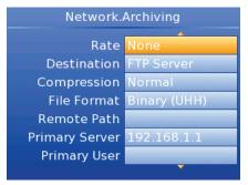
In Network Archiving configure the 'Destination' to 'FTP Server'and 'File Format' to 'Binary (UHH)' \*.
