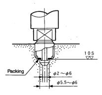
3.3 Apply tightening torque, referring to the table below. To mount or dismount, apply a spanner to the bevelled edge (14mm in width) on the connecting screw section.
