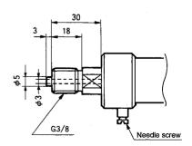
3.2 Mount the transducers as illustrated below. Use a new packing.
