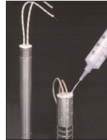
Ceramacast™ 586 pots ignitor and cartridge heater.
