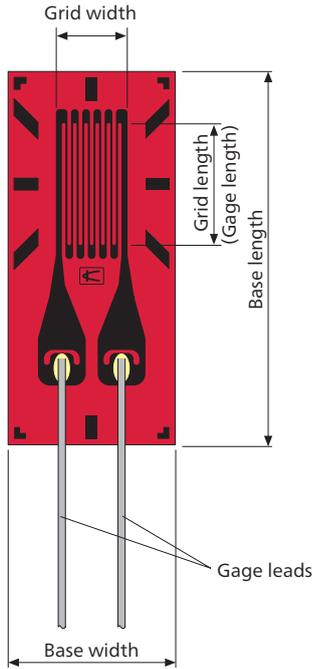
The KFGS series gages use polyimide resin for the base part that is approx. 13  $\mu\text{m}$  thick. It ensures excellent flexibility. The outstanding moisture proof enables the KFGS gages to operate in outdoor measurement effectively. Unless directly exposed to water drop, no coating treatment is required.
