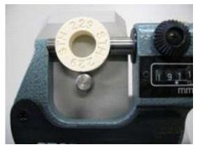
Fig. : Positioning the ring for measurement
