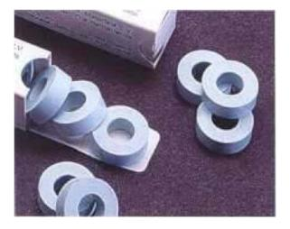
transferred to the ring, by means of conduction, convection and radiation. It takes into account different firing conditions that may occur in a kiln such as heat sinks, temperature gradients, gasflow, heat transfer coefficient, time, kiln setting, etc. Because of total heat measurement, the repeatability of the process is assured and thus so the quality level of the product.
