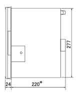
Panel cutout and minimum clearance for installation
