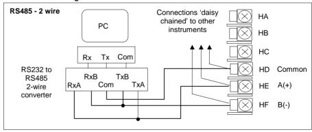
Figure F-12: RS485 2- Wire Communications Connections
