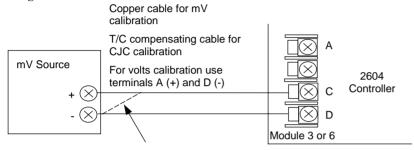
For best results 0mV should be calibrated by disconnecting one of the copper wires from the mV source and short circuiting it to the other wire. This is particularly important to obtain best accuracy for RTD calibration
