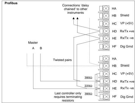
Figure F-14: Profibus Wiring Connections
