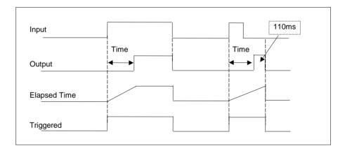
Figure 13-2: Off Delay Timer Under Different Input Conditions
