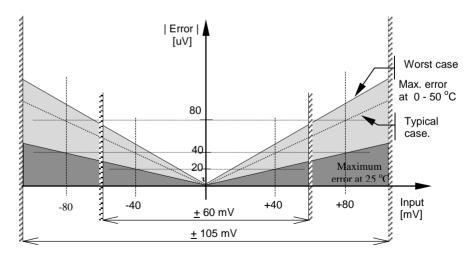
Figure C-1: Error Graph - mV Input
