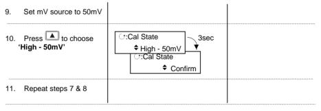
At this point the new calibration values are used by the controller. They will, however, be lost when the power to the controller is turned off. Complete the following step to store the values to the User Calibration area.
