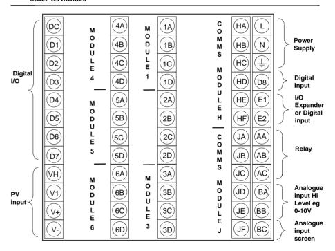
Figure F-3: Rear Terminal Connections
