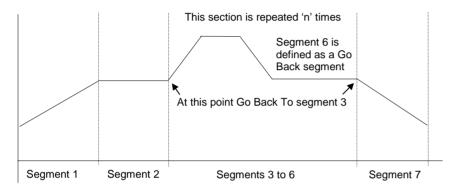
Figure 6-4: An Example of a Program with Repeating Section
