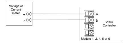
Figure 24-4: DC Module Connections Volts or Current Output
