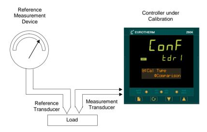
Figure 21-3: Comparison Calibration
