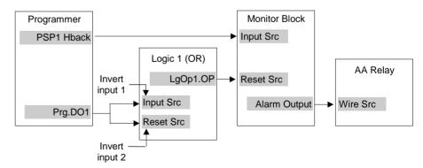
Figure 12-8: Example Wiring, Holdback Duration Timer
