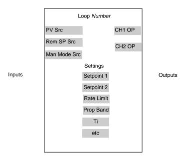
Figure 2-1: A Simple PID Function Block
