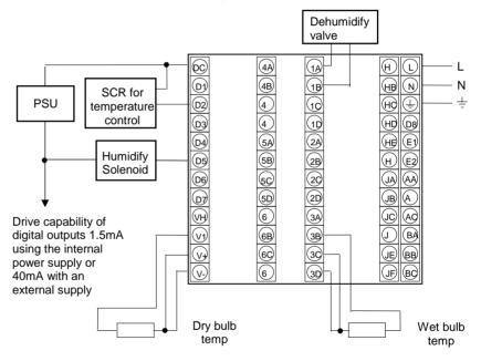
In the above example the following modules are fitted. This will change from installation to installation:
