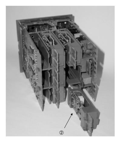
Figure 1-7: View of the Plug-in Modules
