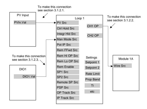
Figure 3-1: A Simple Wiring Example of a PID Function Block
