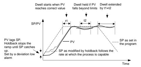
Figure 6-3: Effect of Holdback to Produce Guaranteed soak
