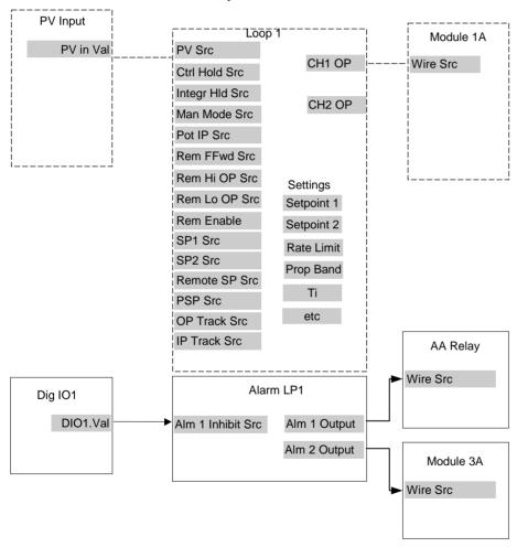
Figure 8-1: Loop Alarm Wiring
