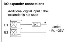
Figure F-8: Wiring Connections for the I/O Expander
