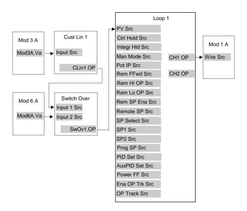
Figure 12-4: Example Wiring, Switch Over Loop with Custom Linearised Input
