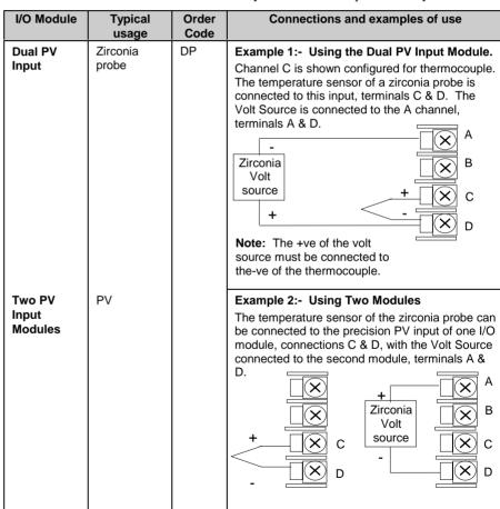
Figure F-16: Wiring Connections for Zirconia Probe
