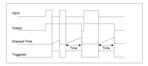
Figure 13-4: Minimum On Timer Under Different Input Conditions
