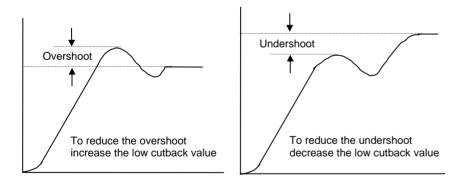
Figure 9-4: High and Low Cutback
