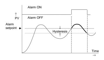
i.e. If the controller is powered up with PV > 'Hi Alarm SP' no alarm is indicated. The PV must reduce below the 'High Alarm SP' and increase again to > 'Hi Alarm SP'. The alarm condition will then be indicated. If the controller is powered up with PV < 'Hi Alarm SP' an alarm is indicated as soon as PV > 'Hi Alarm SP'
