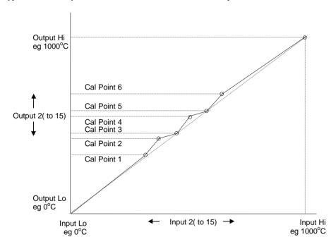
Figure 12-2: Compensation for Sensor Discontinuities
