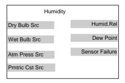
Figure 11-5: Humidity Function Block
