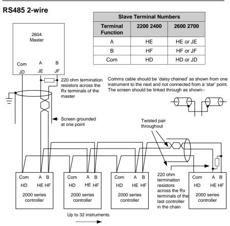
Figure 18-3: Example Wiring RS485 2-wire for 2000 Series Instruments
