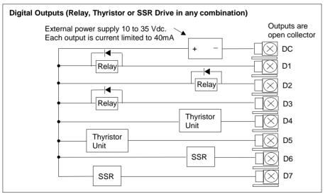
Figure F-10: Wiring Connections for Digital I/O
