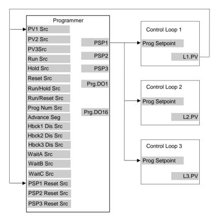
Figure 6-7: Example Programmer Wiring One Profile Three Loops
