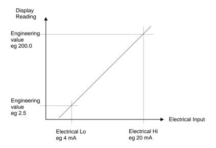
Figure 20-4: Input Scaling (Modules)
