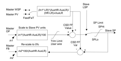
Figure E-1: Cascade Trim Mode - Software Versions Earlier Than V4.0
