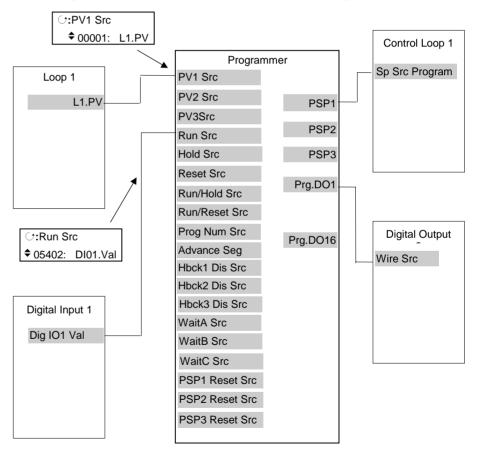
Figure 6-6: Programmer Function Block and Wiring Example
