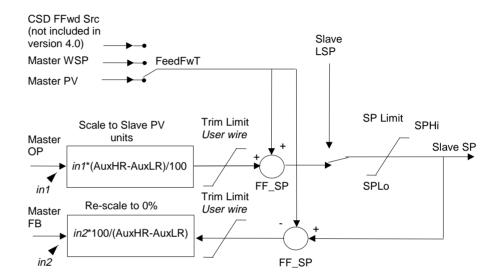
Figure 10-5: Cascade Controller in Trim Mode
