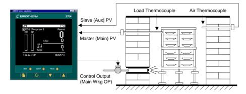
Figure 10-4: Cascade Control of a Furnace Load
