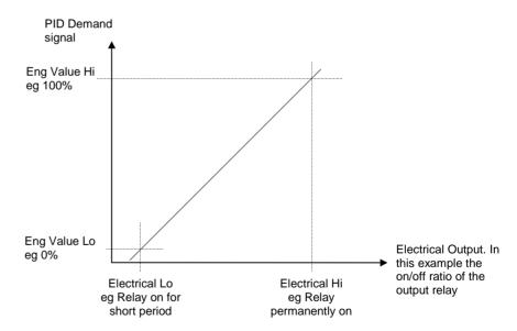
Figure 19-3: Fixed Relay Scaling
