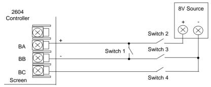
Figure 24-3: Analogue Input Calibration Connections
