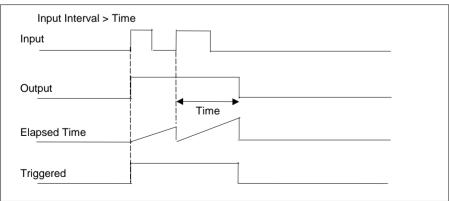
Figure 13-1: On Pulse Timer Under Different Input Conditions
