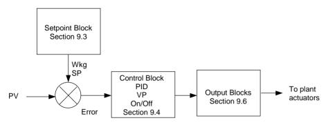
Figure 9-1: Single Loop Controller
