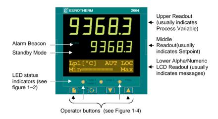
Figure 1-3: Operator Interface
