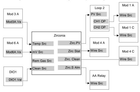
Figure 11-3: Zirconia Wiring for Carbon Potential
