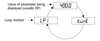
Figure 10-1: Display of Tuning State (Middle Display)
