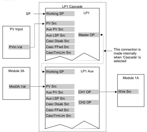
Figure 9-10: Wiring for Simple Cascade Control Loop
