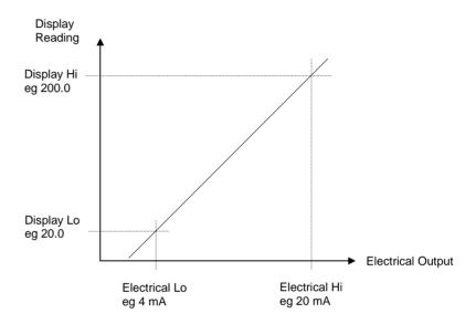
Figure 20-6: Scaling a Retransmission Output
