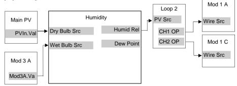
Figure 11-6: Humidity Control Loop
