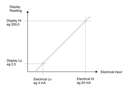
Figure 19-2: Input Scaling (Standard IO)
