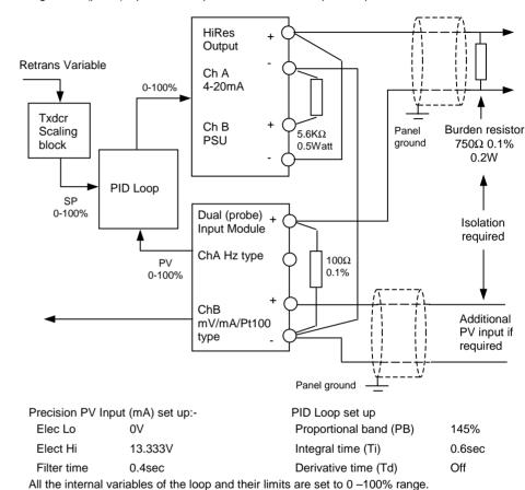
Channel C input and the retransmitted 4-20mA output must be connected together at the (-) terminal of the Dual (probe) input. The receiving instrument 4-20mA input and the other end of the channel C input should be isolated from each other. It is the installers responsibility to ensure the appropriate isolation when using the Dual (probe) module.
