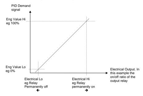
Figure 20-5: Time Proportioning Relay, Triac or Logic Output
