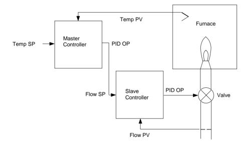
Figure 9-6: Full Scale Cascade Control
