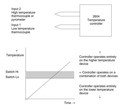
Figure 12-3: Thermocouple to Pyrometer Switching
