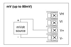
Figure F-6: Wiring Connections For PV Input
