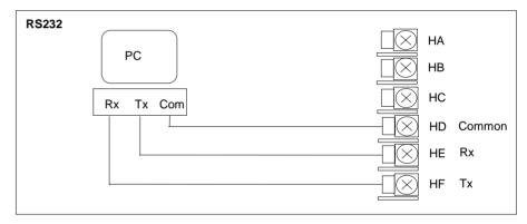
Figure F-11: RS232 Communications Connections
