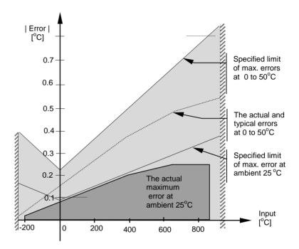
Figure C-4: Error Graph - RTD Input
