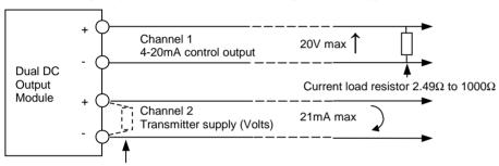
A resistor of approx  $56K\Omega$  should be added if the current load <0.5mA
