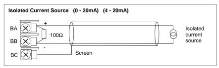
Figure F-7: Wiring Connections For Analogue Input
