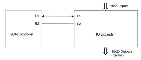
E1 and E2 are the terminal numbers on both Controller and IO Expander. It is recommended that a cable length of 10 metres is not exceeded, however, no shielding or twisted pair cable is required.
