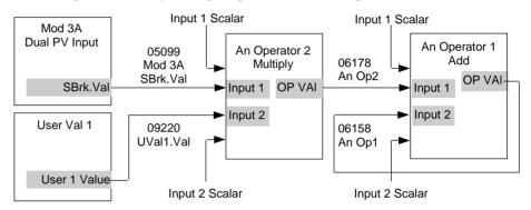
1. In MODULE set 'SBrk Impedance' = High IO/Module 3A (or 6A)
