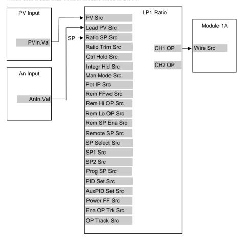
Figure 9-12: Wiring for Simple Ratio Control Loop
