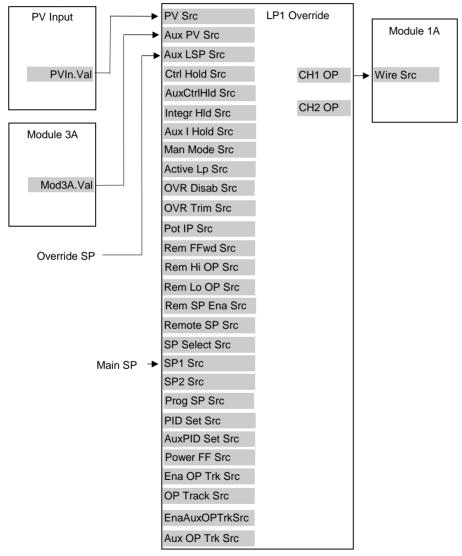
Figure 9-14: Wiring for Simple Override Control Loop
