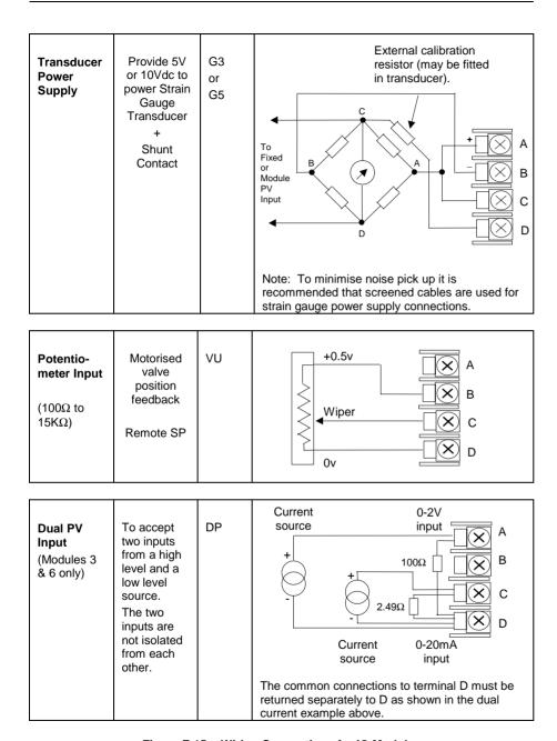
Figure F-15: Wiring Connections for IO Modules
