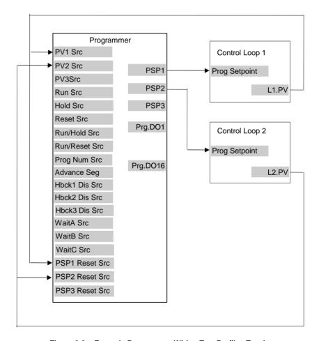
Figure 6-8: Example Programmer Wiring Two Profiles Two Loops
