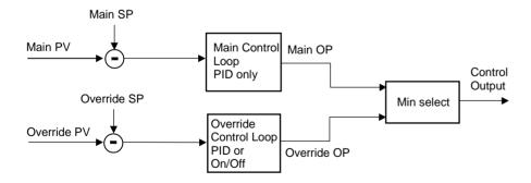
Figure 9-13: Simple Override Control (Select Minimum)
