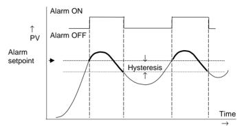
Hysteresis is the difference between the alarm ON value and the alarm OFF value. It is used to prevent relay chatter.
