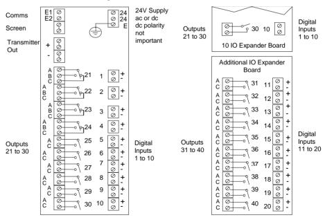
Figure F-9: IO Expander Connections
