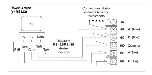
Figure F-13: RS485 4-Wire Communications Connections
