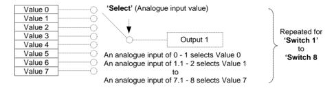
Figure 14-3: Representation of an Analogue Switch
