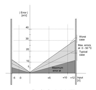
Figure C-3: Error Graph - 0 - 10V Input
