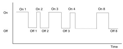
Figure 7-1: An Example of a Programmed Digital Output
