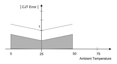
Figure C-5: Overall CJT Error at Different Ambient Temperatures
