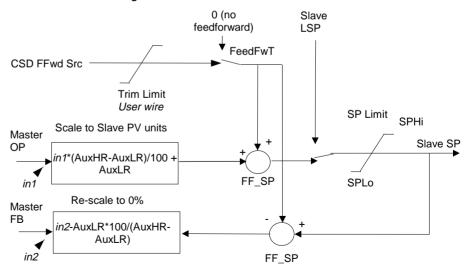
Figure 9-9: Cascade Controller in Full Scale Mode
