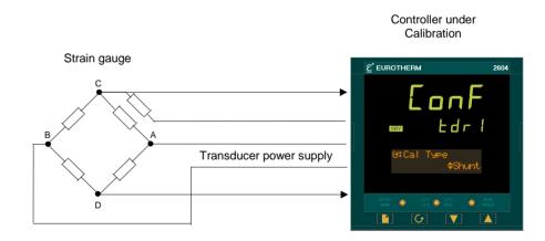
Figure 21-1: Strain Gauge Calibration
