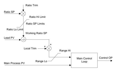
Figure 9-11: Simple Ratio Control Block Diagram
