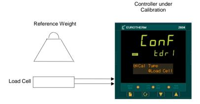
Figure 21-2: Load Cell Calibration
