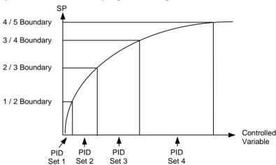
Figure 9-5: Gain Scheduling in a Non-Linear System
