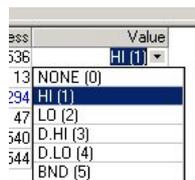
4. Select the alarm type - in this example HI. (1) is the enumeration of the parameter.
