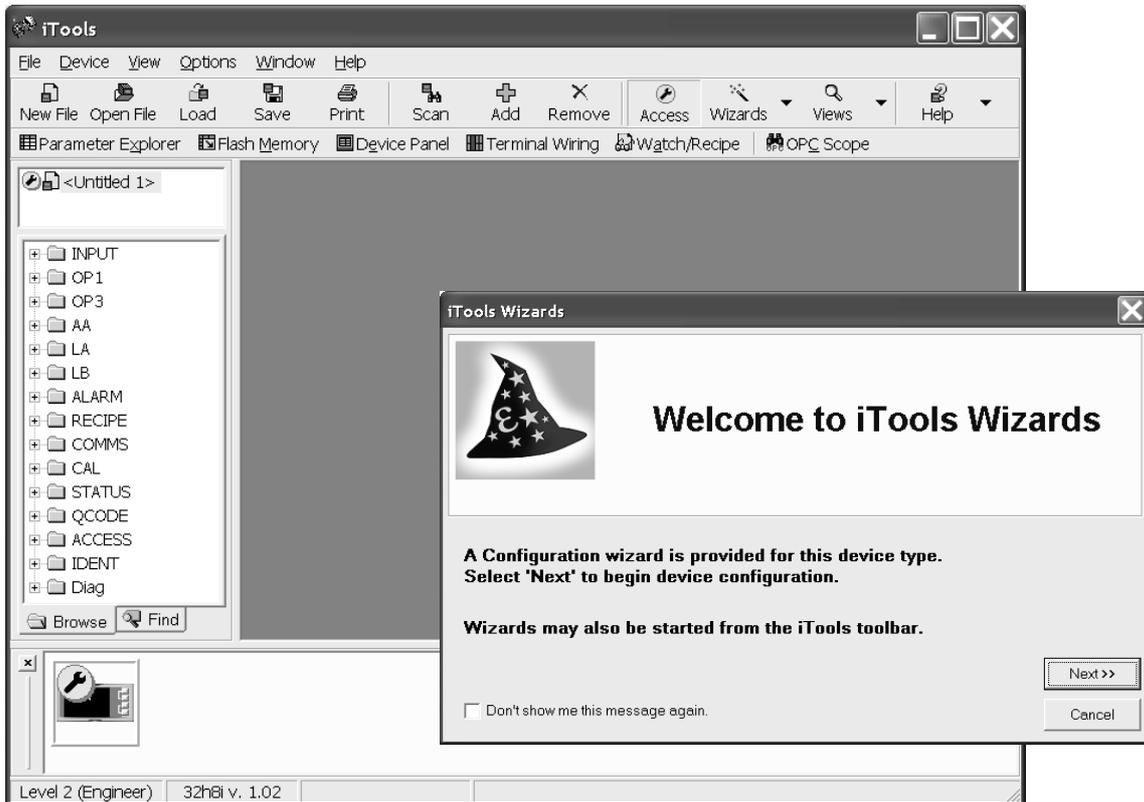
The instrument may be configured using a **Wizard** or from the browser view. The following pages show a number of examples of how to configure various functions using either of these features.
