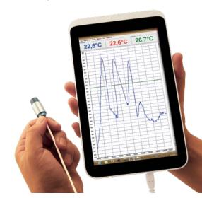
A **complete parameter set-up** is also supported. Thanks to the use of modern tablet PCs this can be done locally where the sensor is installed. This feature includes, for example, the adjustment of the sensor's measuring parameters (emissivity, offsets, alarm threshold) or the possibility to compensate for the ambient temperature.
