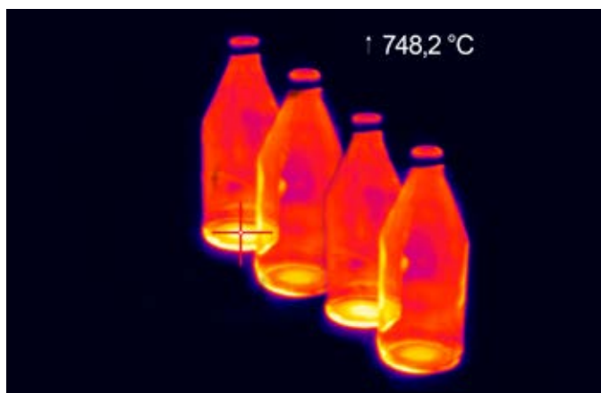
Hot spot detection at glass bottle production
