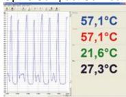
The licence-free temperature analysis software Optris Compact Connect allows simple and fast parameterization of the compact and the high performance series' fixed infrared thermometers. It further serves the analysis and documentation of temperature measurement values, thus optimizing process control.
