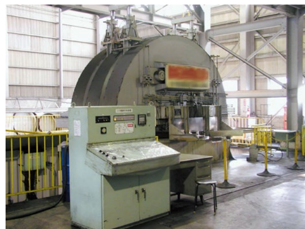
Pressing of isotropic graphite
