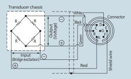
For most transducers, the shield wire is not connected to the case.
