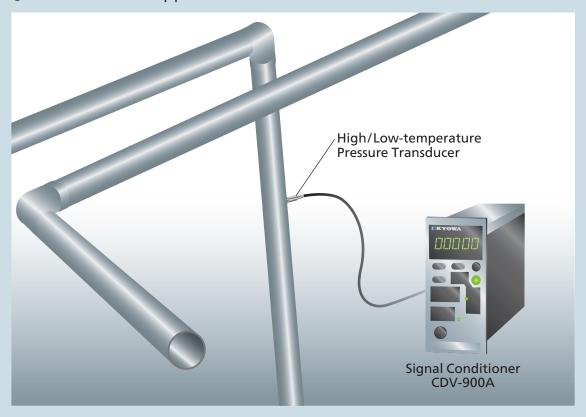
• Refrigerant pressure monitor of air conditioning facilities.
