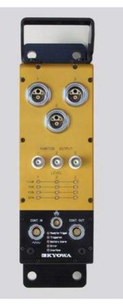
The unit is rated to withstand up to 980.7m/s<sup>2</sup>(100g).
