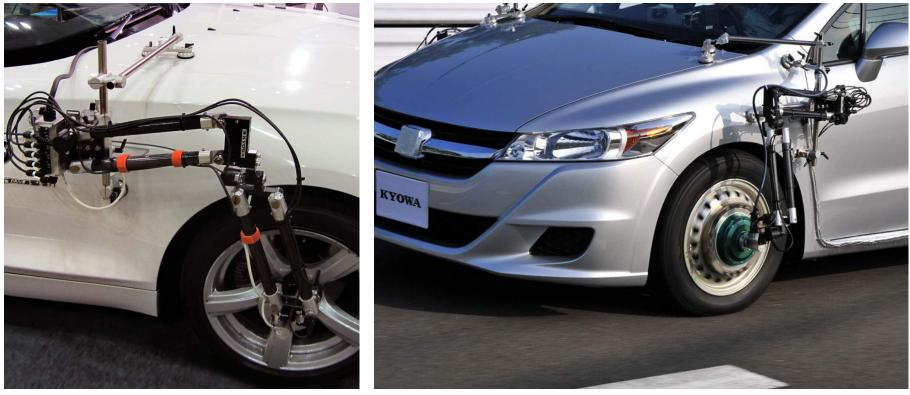
The system can be used independently(left), or with the slip-ring type wheel 6-component force measuring system(right).
