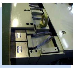
This 48 force sensor matrix is designed for installation on an Offset Barrier Frame. Each of 48 sensor units consists a strain gage type 124mmX124mm load cell to evaluate compatibility.
