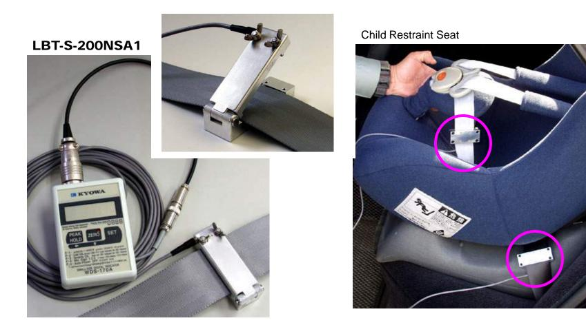
Use for measuring tensile force to install CRS (Child Restraint Seat)
