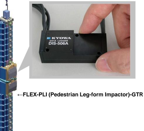
Install 4-units of DIS-506A into FLEX-PLI to make 24channel Measurement.
