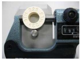
The "T"'s impressed in the ring should be placed exactly on the indentation of the micrometer.
