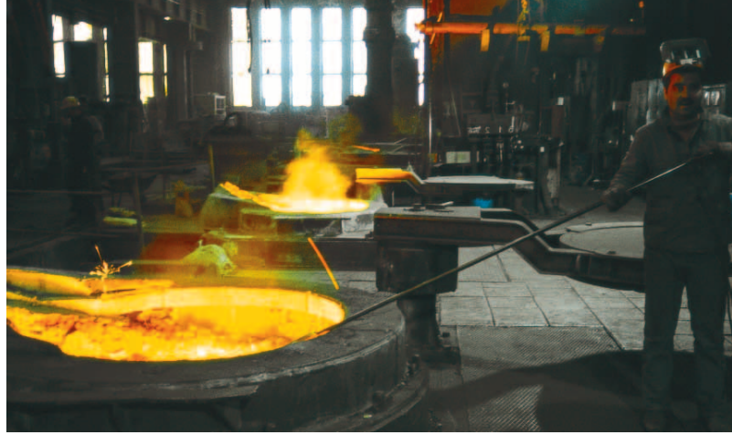
Immersion temperature measurement in cast iron
