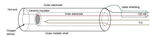
If the probe is situated in an area of high interference, it is preferable to use shielded wires for the voltage source of the probe (oxygen sensor) and the shielding connected to the outer metallic shell of the probe.
