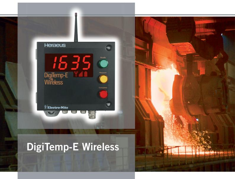
Temperature measurement in molten metals
