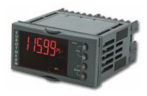
Model number 32h8e is a horizontal 1/8DIN indicator and alarm unit that performs the dual function of remote display for EPower and independent 'policeman'. The latter is intended to disconnect should an overtemperature (or other excess process condition) occur. 32h8e communicates with EPower using Modbus protocol via the EIA485 RJ45 connector located on the underside of the EPower controller.
