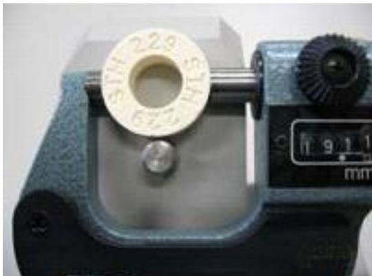
Fig. : Positioning the ring for measurement
