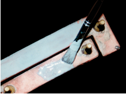
Cerabond™ 571 coats copper induction heater.
