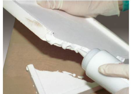
Cerabond™ 503 repairs furnace saggar plate.
