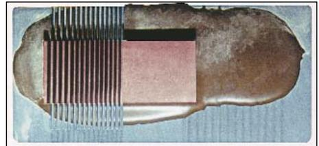
Crystalbond™ 590 bonds an advanced ceramic which is diced into 25-50 mil sections.
