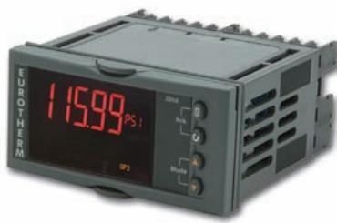
Model number 32h8e is a horizontal 1/8DIN indicator and alarm unit that performs the dual function of remote display for EPower and independent 'policeman'. The latter is intended to disconnect should an overtemperature (or other excess process condition) occur. 32h8e communicates with EPower using Modbus protocol via the EIA485 RJ45 connector located on the underside of the EPower controller.
