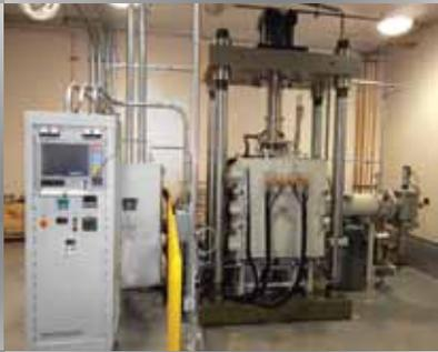
Model HP500-242424G provides 250 tons of force, a spacious 24" cube usable work space, 4-side graphite hot zone rated at 1800° and operates in inert gas, vacuum or a partial pressure environment.
