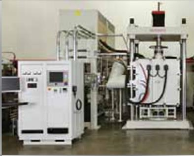
Diffusion bonding hot press operating at 1450°C with a total force of 100 tons. The 24"x24"x30" molybdenum hot zone is capable of diffusion bonding multiple parts in one load. System footprint measures approximately 9 1/2' wide, 15' deep and 12 1/2' high.
