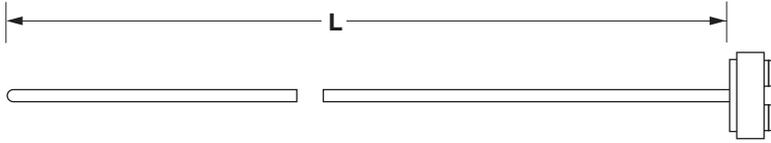
The Style AS thermocouple features a “wafer” head, which allows quick access to terminal screws for wiring. This thermocouple is an economical choice because the termination is attached directly to the XACTPAK sheath.
