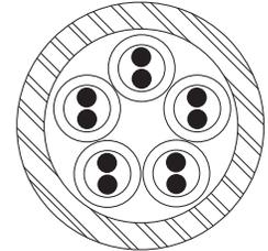
Thermocouple sensors made from mineral insulated, metal-sheathed cable are positioned inside the overall protection sheath.
