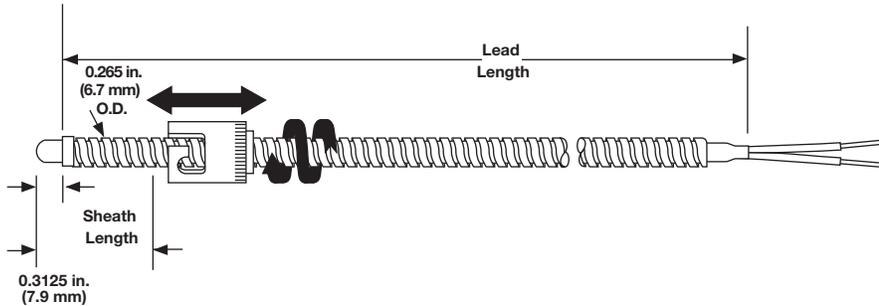
Adjustable armor thermocouples bend to any angle to fit a wide range of hole depths, eliminating the need to stock numerous styles. A stainless steel hose offers additional lead protection in demanding applications.
