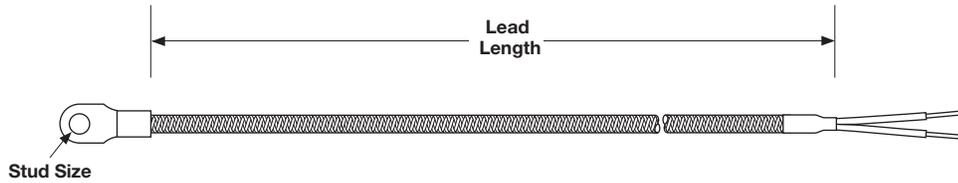
The nickel terminal can be placed beneath existing screws or bolts to permit surface temperature measurement.
