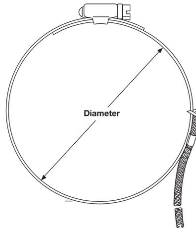
The stainless steel clamp allows temperature measurement without drilling or tapping which is ideal for measuring pipe temperatures.
