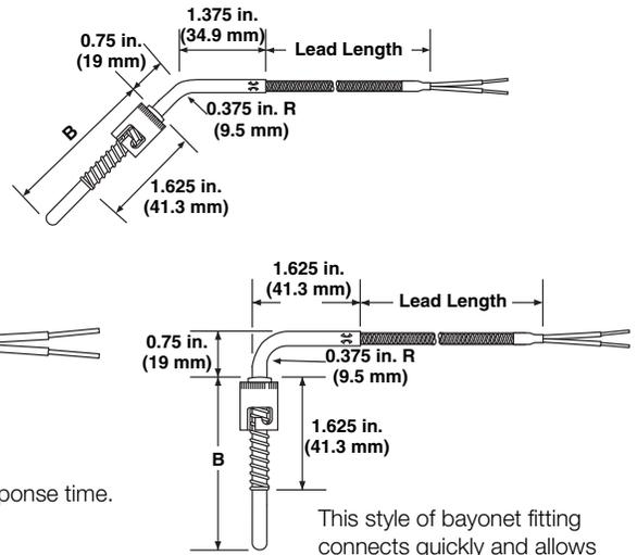
This style of bayonet fitting connects quickly and allows leads to exit with a protective sheath.
