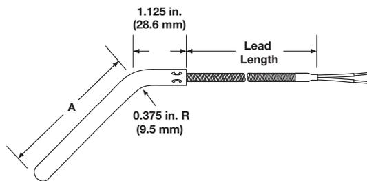
The bent rigid tube offers protection and accurate lead placement around machinery.
