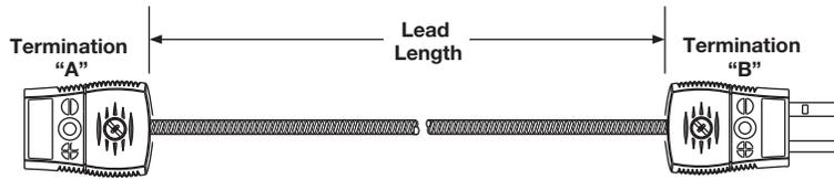
Flexible extensions allow thermocouples to be disconnected from a system without disturbing the remaining wiring.
