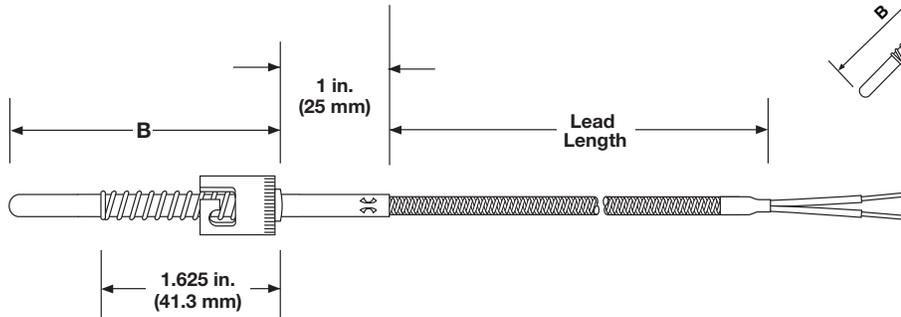
Bayonet fittings allow rapid attachment. Spring pressure on the junction tip assures fast response time.
