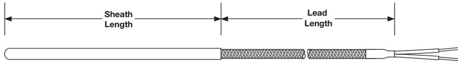
The rigid sheath is covered with a 0.010 in. (0.25 mm) wall of PFA for corrosion resistance in acid environments. An epoxy seal improves moisture resistance of the sensor and provides a barrier for migrating fumes in corrosive applications.
