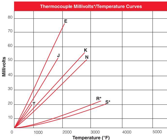
\*Millivolt values shown for R and S calibrations pertain to thermocouple calibrations only. RX and SX constructions described in this catalog section are intended for use as **extension wire only** and will not exhibit the millivolt outputs shown.
