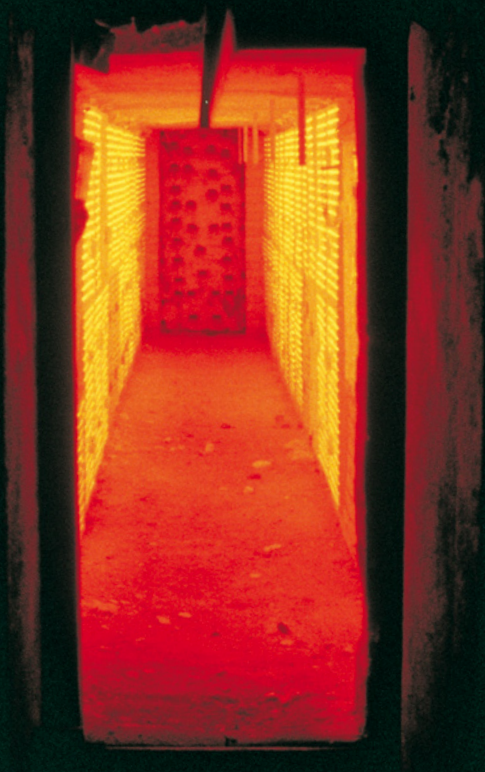
Fig. 31. FIBROTHAL modules in a suspended monorail furnace
