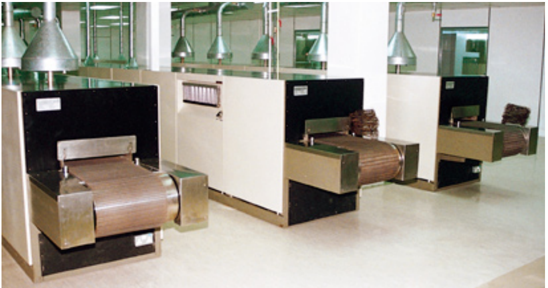
Fig. 32. FIBROTHAL modules used in a conveyor belt furnace
