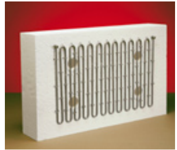
Fig. 3. MEANDERTHAL II module with free-radiating heating elements for a maximum element temperature of 1300°C, mainly for roof heating and tilting furnaces
