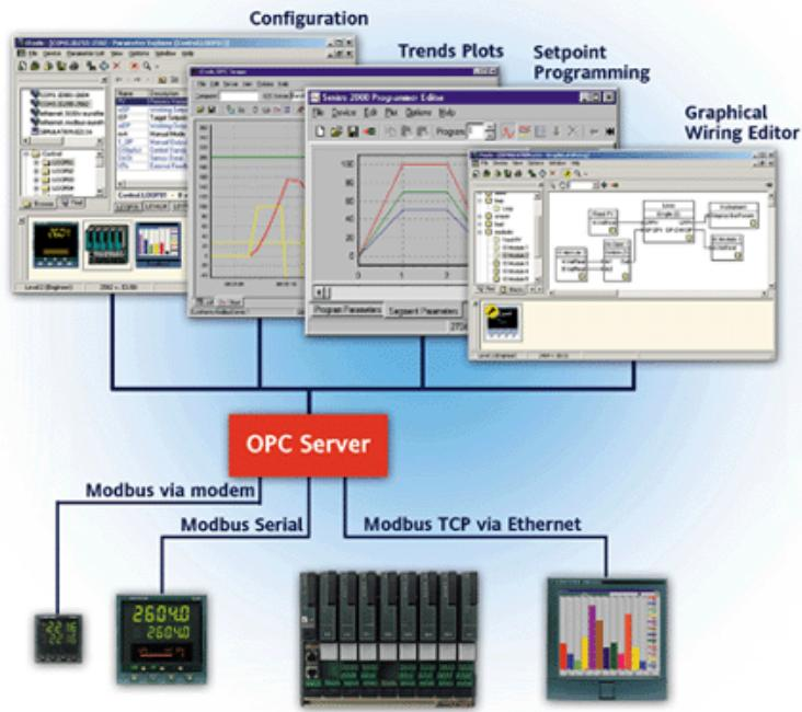
iTools is a Windows based software package designed for configuration and cloning of the industry leading Series 2000™ family of PID controllers and indicators. With iTools V4 or greater there is support for the Chessell 5000 Series of graphical DAQ recorders. There are 3 editions of iTools - Demo, Standard and Open. The Demo edition of iTools may be downloaded free from the Eurotherm web site for evaluation.
