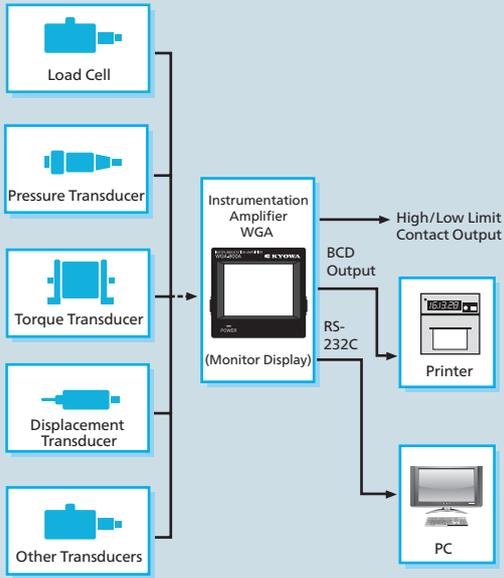
Transducer's connectors and cables differ depending on models. For details, refer to description of each model or page 8-1.
