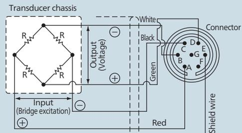
For most transducers, the shield wire is not connected to the case.
