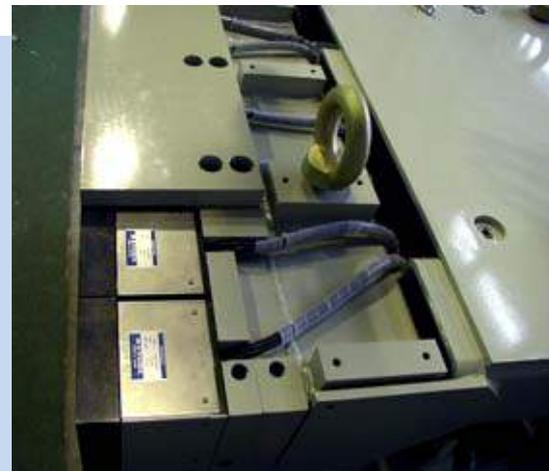
This 48 force sensor matrix is designed for installation on an Offset Barrier Frame. Each of 48 sensor units consists of a strain gage type 124mmX124mm load cell to evaluate compatibility.
