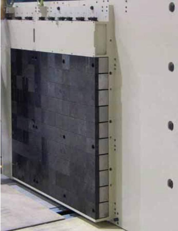
◆ This 160-channel force sensor array mounts directly on the front barrier wall to measure Impact force distribution.
