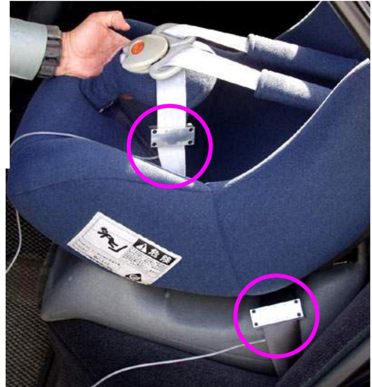
**Use for measuring tensile force to install CRS (Child Restraint Seat)**
