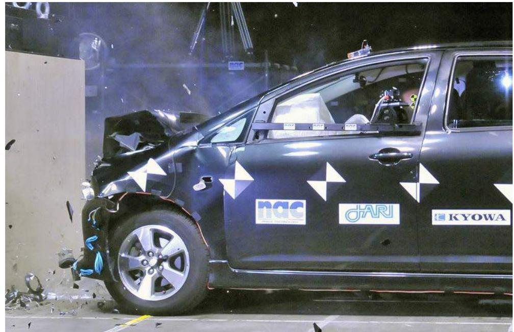
◆ Each force sensor consists of strain gage-based load cell, and measure impact forces.
