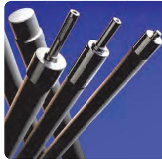
Their outstanding mechanical properties and special surface finish make our fused silica rollers indispensable as transport rollers in all kinds of glass tempering furnaces. These furnaces are used to finish e.g. safety glass for use in architecture and the automotive industry. Furthermore, we also offer fused silica rollers with integrated metal end caps in many designs. Customised shapes do not present any problems.
